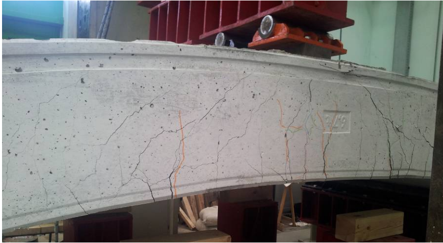
Figure 34. Segment D5: failure stage: right lateral surface.
