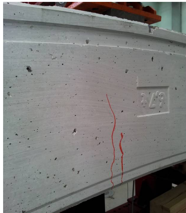
Figure 12. Segment D4: load level of 175 kN; a) left lateral surface, b) right lateral surface
