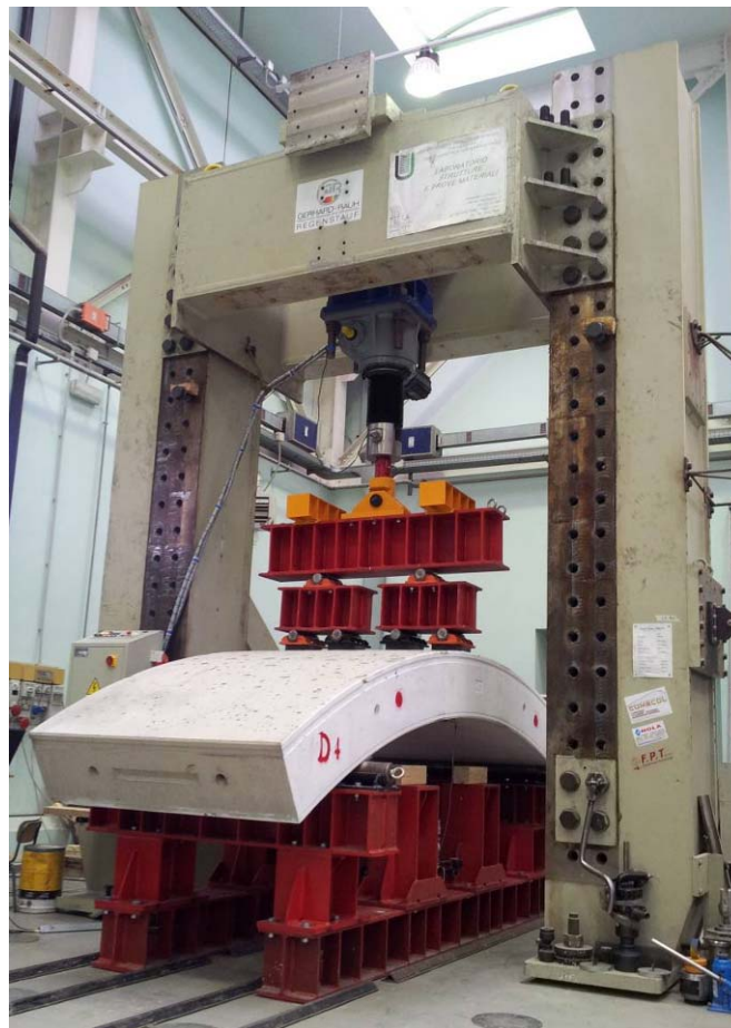
Figure 5b. Bending test set-up
