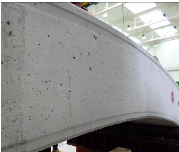
Figure 12. Segment D4: load level of 175 kN; a) left lateral surface, b) right lateral surface
