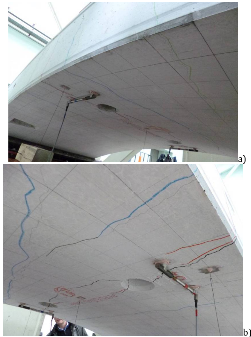
Figure 18. Segment D4: load level of 300 kN – intrados surface; a) left side; b) right side
