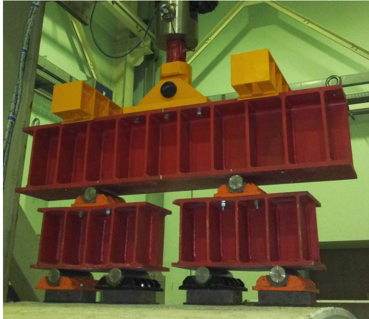
Figure 7. Loading distribution system
