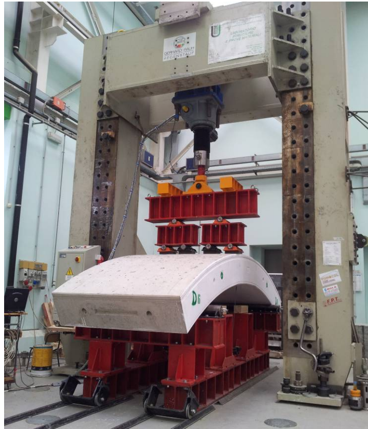
Figure 38. Segment D6: Test set-up
