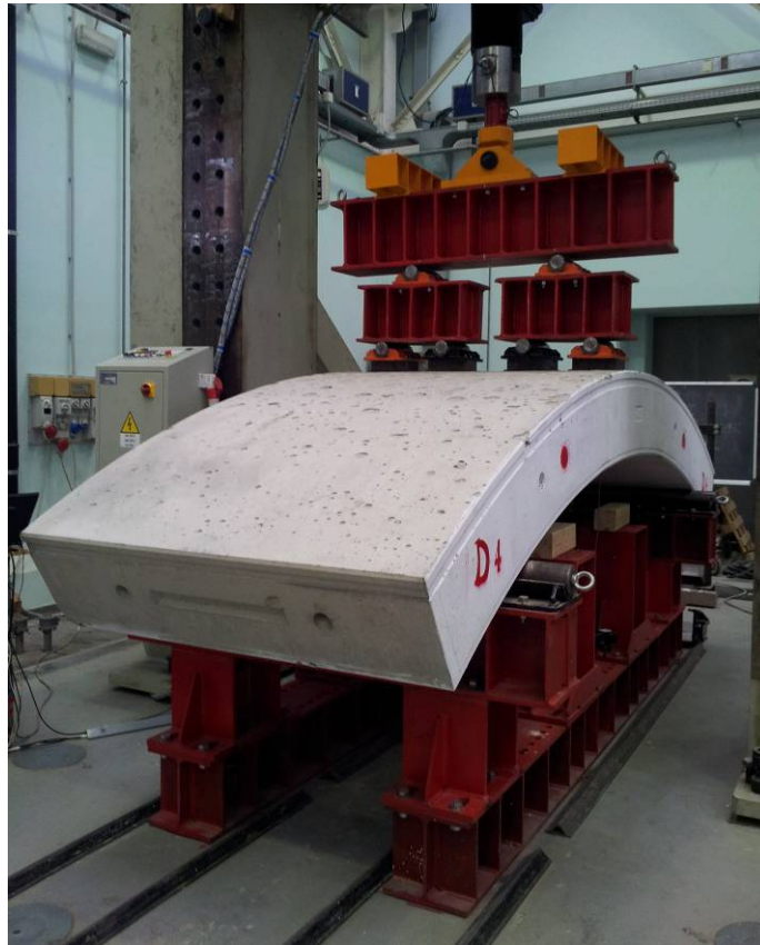
Figure 10. Segment D4: Test set-up
