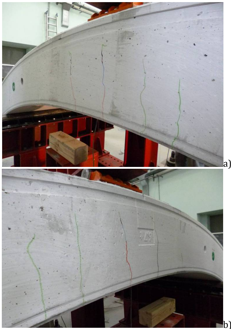
Figure 45. Segment D6: load level of 185 kN; a) left lateral surface, b) right lateral surface.
