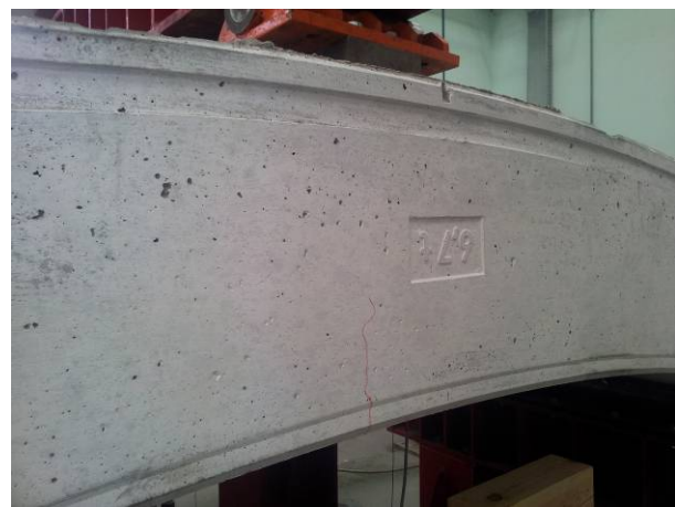
Figure 26. Segment D5: load level of 130 kN; a) left lateral surface, b) right lateral surface
