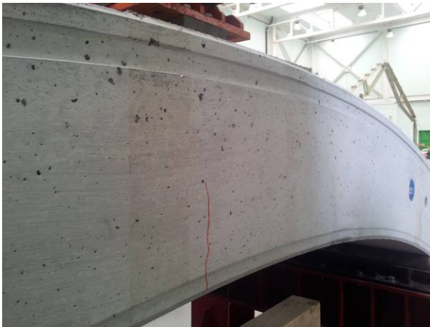
Figure 26. Segment D5: load level of 130 kN; a) left lateral surface, b) right lateral surface
