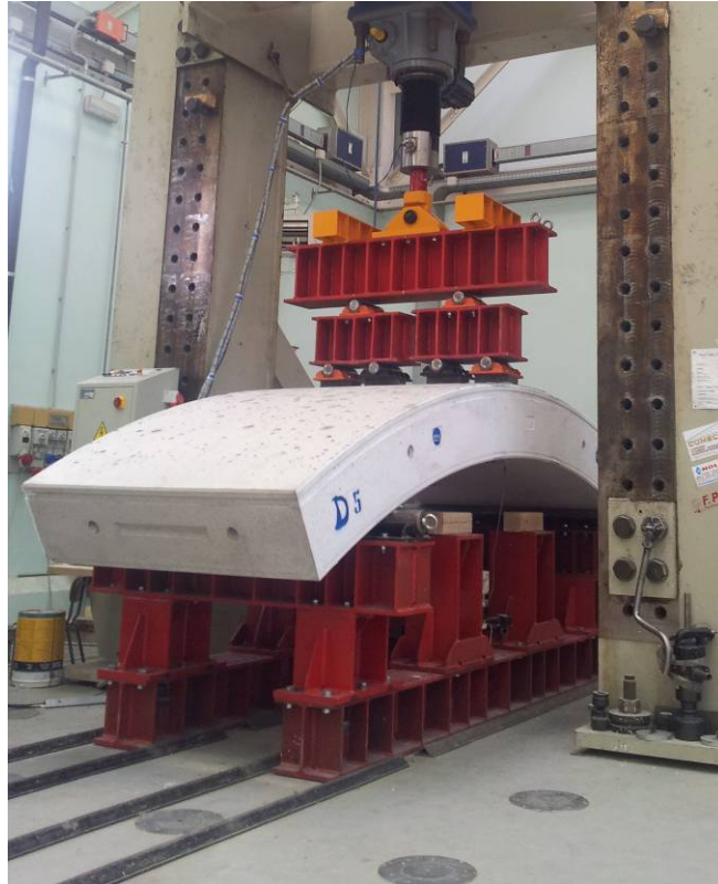
Figure 24. Segment D5: Test set-up
