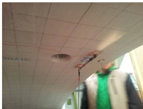
Figure 27. Segment D5: load level of 130 kN intrados surface(a); b) left side; c) right side
