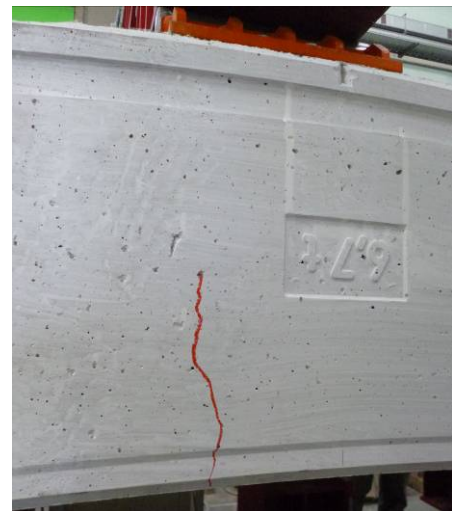
Figure 40. Segment D6: load level of 140 kN; a) left lateral surface, b) right lateral surface
