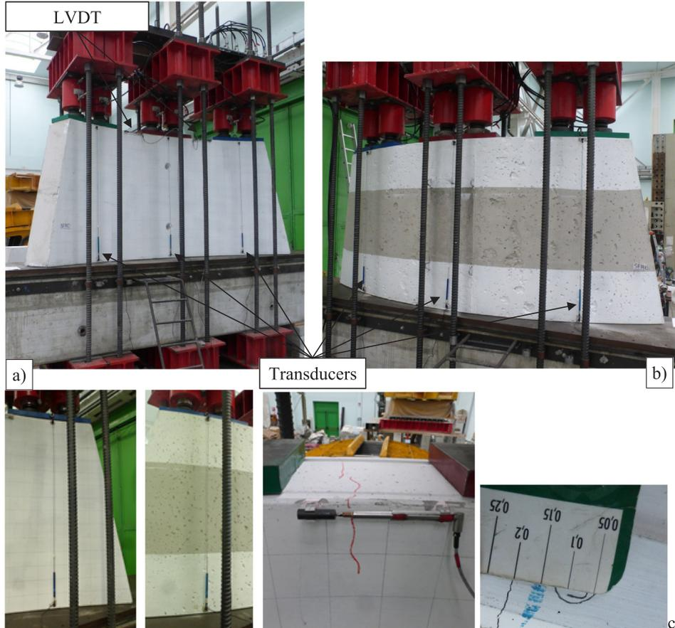
Fig. 7. Point load test and instrumentation: (a) Intrados surface; (b) Extrados surface; (c) detail of the potentiometer transducers, LVDT device and crack gauge.
