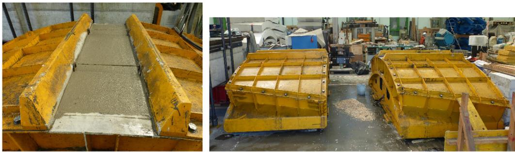
Fig. 2. Segment cast and curing.
