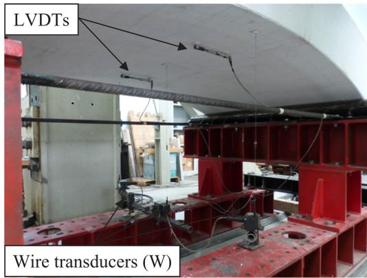
Fig. 6. Bending test instrumentation.
