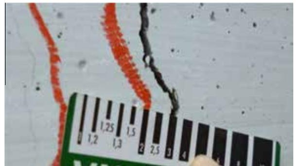
Fig. 11. Segment SR: load level of 300 kN, maximum crack width (lateral surface).
