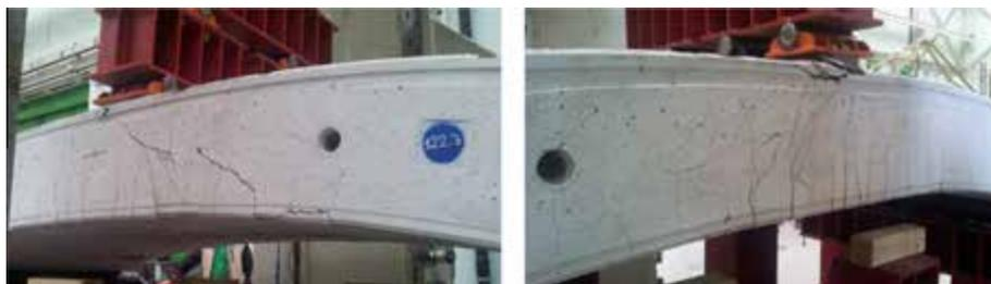
Fig. 22. Segment GFR: failure stage - right lateral surface.
