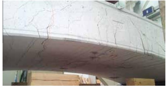
Fig. 23. Segment GFR: failure stage - intrados surface.
