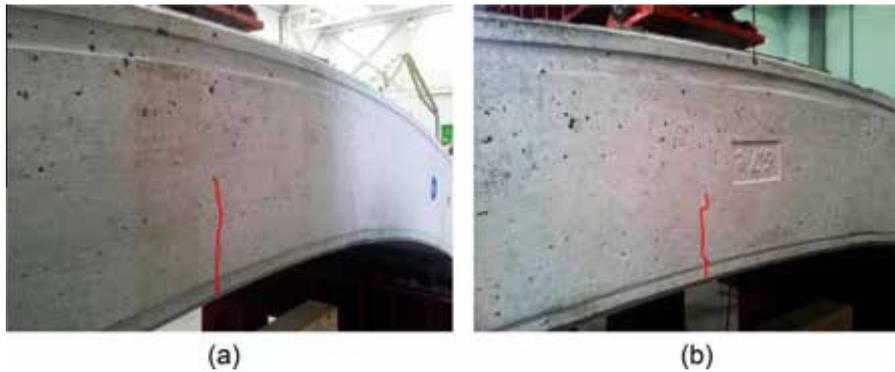
Fig. 17. Segment GFR: load level of 130 kN; (a) left lateral surface and (b) right lateral surface.
