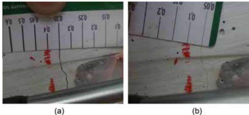
Fig. 33. Second cycle: maximum crack width; (a) load level 2500 kN; (b) complete unloading.
