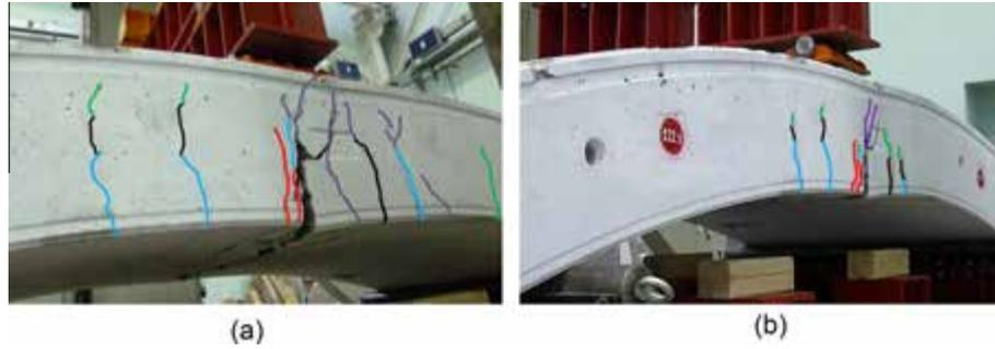
Fig. 12. Segment SR: failure stage (a) left lateral surface and (b) right lateral surface.
