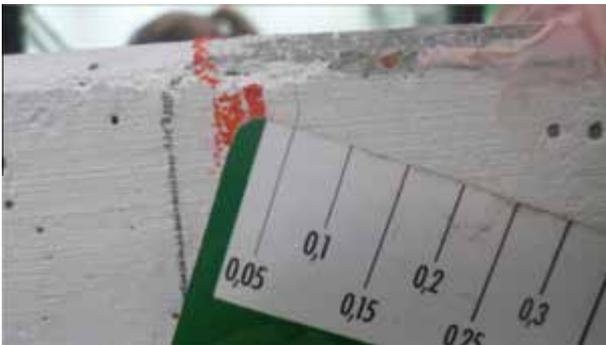
Fig. 31. First cycle. Maximum crack width (1130 kN).
