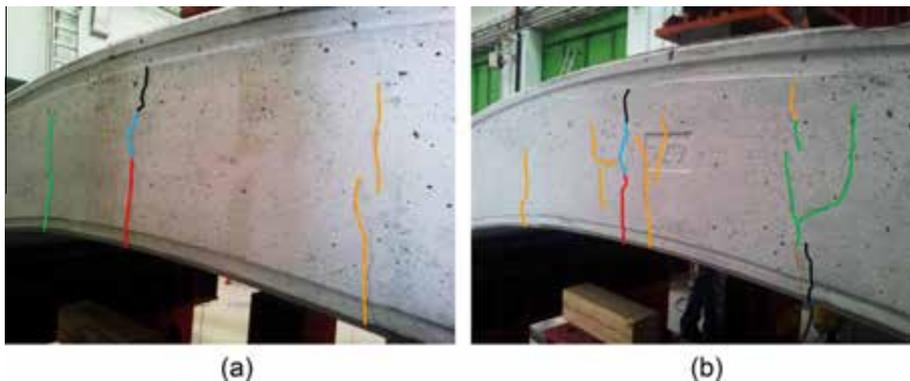
Fig. 19. Segment GFR: load level of 195 kN; (a) left lateral surface and (b) right lateral surface.
