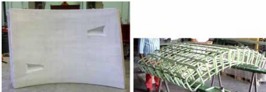
Fig. 28. Segment geometry for the TBM thrust test.
