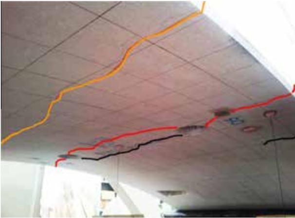
Fig. 20. Segment GFR: load level of 195 kN - intrados surface.
