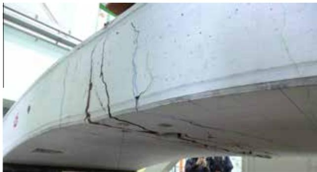
Fig. 13. Segment SR: failure stage - intrados surface.
