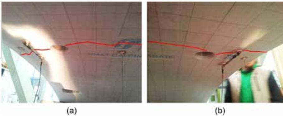
Fig. 18. Segment GFR: load level of 130 kN. Intrados surface: (a) left side and (b) right side.
