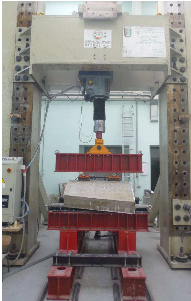
Figure 4. Bending test set-up
