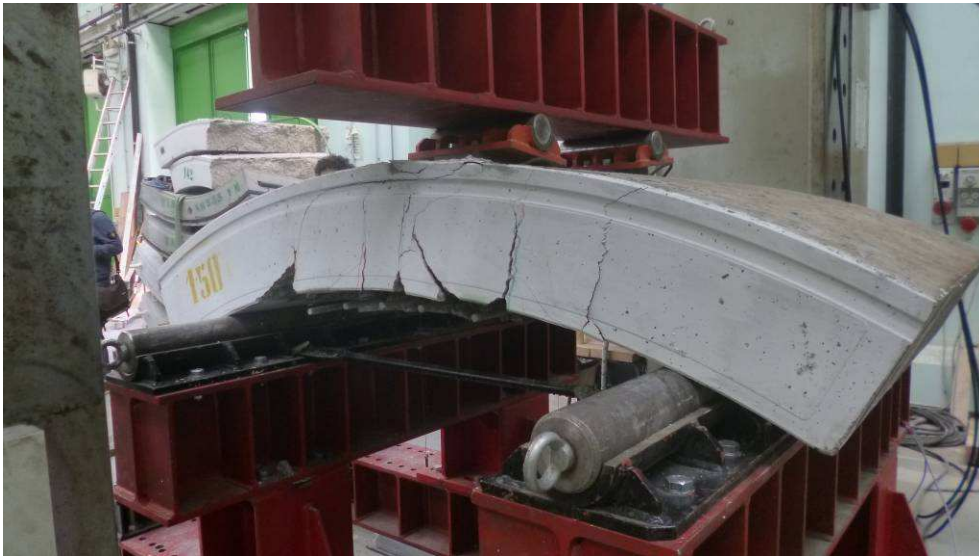
Figure 13. Failure condition right lateral surface
