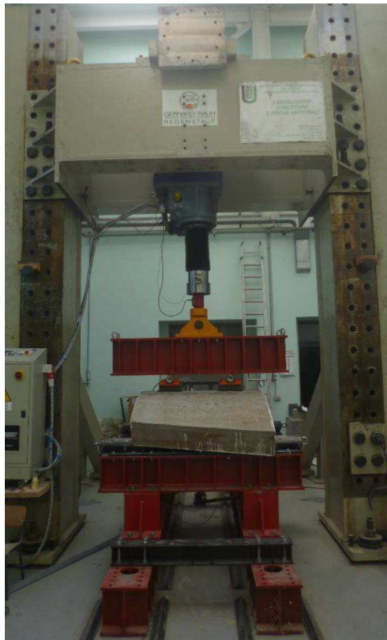
Figure 6. Segment 150: Test set-up
