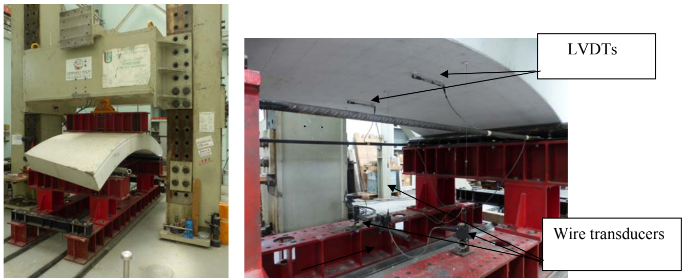
Figure 4. Bending test set-up and instrumentation
