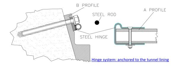
Furthermore, in order to avoid the unintentional reclining of GFRP "A" profile (e.g. during metro traffic), it is possible to lock it by means of security lock as in figure.
