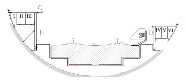
In detail, there are three wiring spaces (I=73082mm², II=118782 mm² and III= 118133 mm²) under the safety walkway for signaling, telecom, fiber optic and low voltage power supply, and three wiring spaces (IV=81275mm², V=81883 mm² and VI=75575 mm²) under the walkway of district cooling pipes for MV-TPS and MV-SPS cables.
