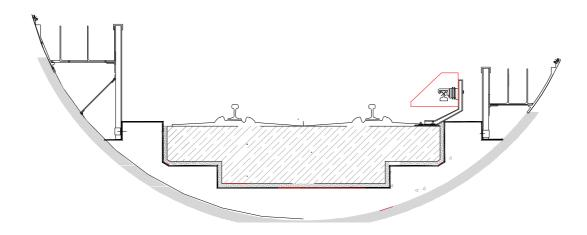
4. Positioning the walkable GFRP type A and A' profiles:
