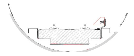
2. Fixing GFRP profiles type G and G' in the soil (after pre-assembling type D,E,F,G,K and I profiles):
