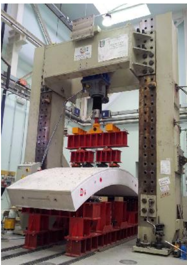
Figure 4 - Bending tests (a). Displacement measuring (b).
