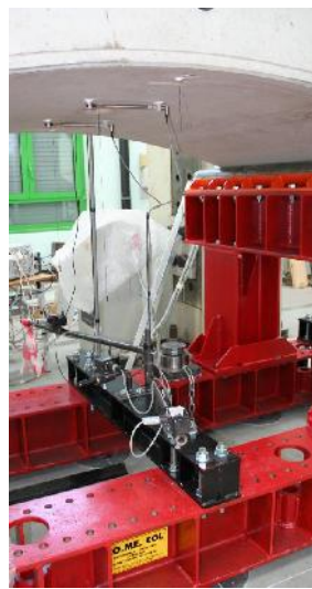
Figure 4 - Bending tests (a). Displacement measuring (b).
